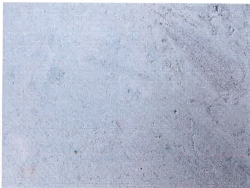
Photo 1: macroscopic look of the POORLY WASHED BIOSPARITE commercially named "Ramon Grey – Grey Gold", (Stereomicroscope 10m)
