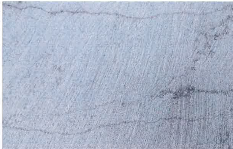
Photo 1: macroscopic look of the DOLIMITIZED INTRA-SPARITE commercially named "Galilee Grey". (Stereomicroscope 10m)
